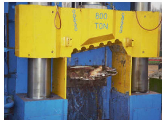
Pic. 4: View on the shear head with cylindric guides (guide covers removed)
