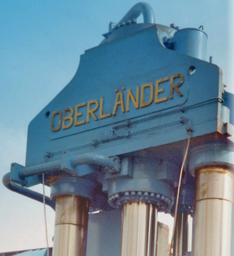
Pic. 1: 800 t Scrap Shear, Type Hy-PS 800
