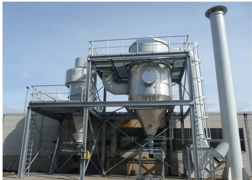
Fig.4: explosion proof exhaust filtering unit
